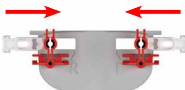
1. Push the lower parts of the tension shoe on the left and right into the recess on the side of the installation aid or press them in from below.
