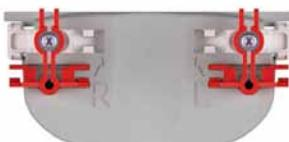
3. By opening the clasp slightly, the screws will fall securely into the screw guide and can then be installed in this position overhead in the upper window rebate as well.
