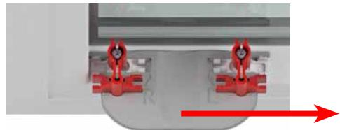
5. When the screw is firmly tightened, slide the fitting template down from the tension shoe to the centre of the window.
