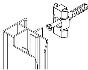
End stop pin guide assembly intermediate guide
