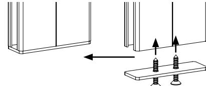
Fitted with an end stop in black plastic or end plate in aluminium at the bottom end to stop the bottom lath; thickness 2 mm.
