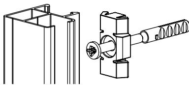
End stop pin guide assembly intermediate guide
