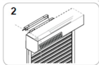
Batteries are always placed outside - not inside the box - for all box sizes.
