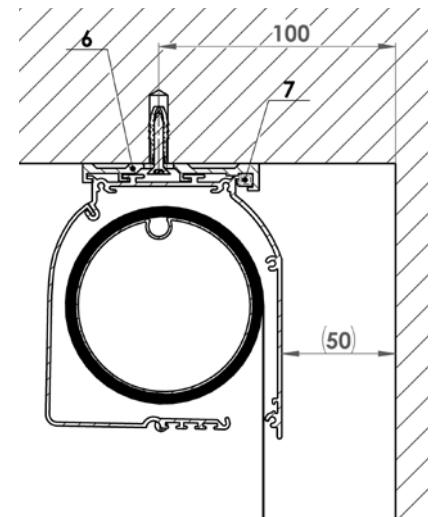
Insert the upper box to brackets (6) and slide it lengthwise until it is centred within the window wing, and secure with wedges (7).
