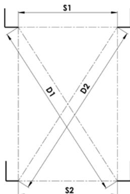
Once the assembly is finished, check parallelism and rectangularity of the guide bars. This can be done by measuring two distances "S1" and "S2" or diagonals "D1" and "D2". The dimensions must be the same  $\pm 2$  mm. Proper guide bar placement is vital, otherwise the function of the roller blind can be impaired. For front guide bar installation, self-adhesive covers are supplied to cover the attachment screw holes.
