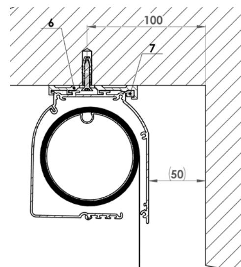
Insert the upper box to the brackets and slide it lengthwise until it is centred within the window wing, and secure with wedges (7).
