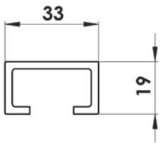
First, attach the box to the ceiling/wall, then install the guide rails. For model GW, only one type of guide rails is available – GC20.
