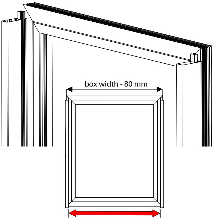
distance between guide rails = box width – 80 mm
