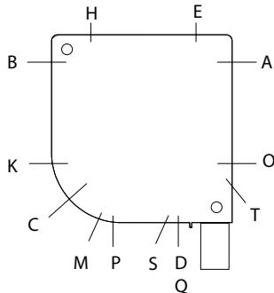
Various exits are possible depending on the operation. The exact location of the operation exit can be seen on the drawings. Consult these drawings before the installation.
