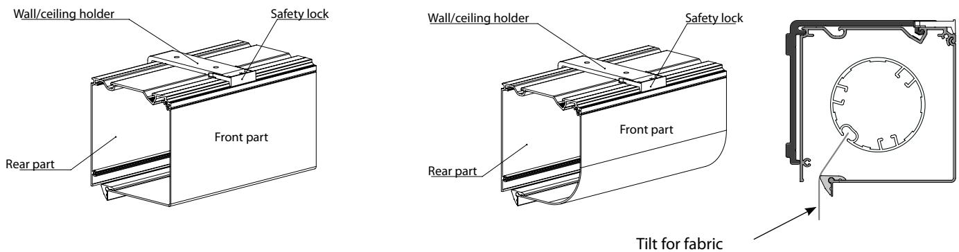
**Material:** extruded aluminium with powder coating finish
