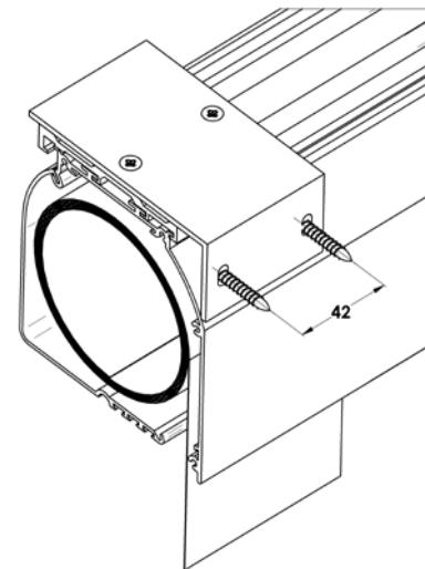
Attach brackets using screws and components suitable for the type of structure onto which they are to be attached (metallic structure, window frame, wall, other material). If four brackets are used, ensure that the brackets are perfectly aligned  $\pm 1$  mm; this can be checked by sliding the box along the cut-outs before tightening the attachment screws. Insert the box to brackets and slide it lengthwise until it is centred within the window wing, and secure with wedges.
