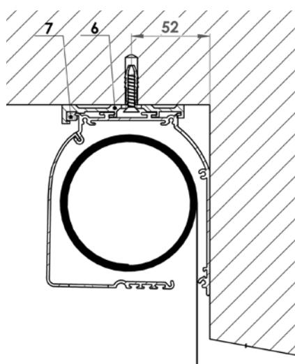
Attach brackets (6) using screws and components suitable for the type of structure onto which they are to be attached (metallic structure, window frame, wall, other material). If three or more brackets are used, ensure that the brackets are perfectly aligned  $\pm 1$  mm; this can be checked by sliding the box along the cut-outs before tightening the attachment screws.
