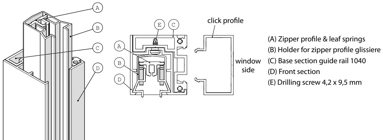
The complete wide 1040 guide rails are made up of a base section (C), a front section (D) and a holder (B) with zipper profile (A), and at the bottom of the base section of each guide rail an aluminium end cap. The front section is fixed into the base section of the guide rail by the drilling screw (see figure). The holder and the zipper profile can only be inserted when the front section is fixed. This is because the holder and the zipper profile are 35 mm longer than the guide rail.
