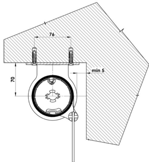
The rolling unit is to be seated at the motor side to HiPro clamp (7) and secured by a lock, while, on the opposite side, the unit is inserted in plastic housing (12) and secured by a screw.
