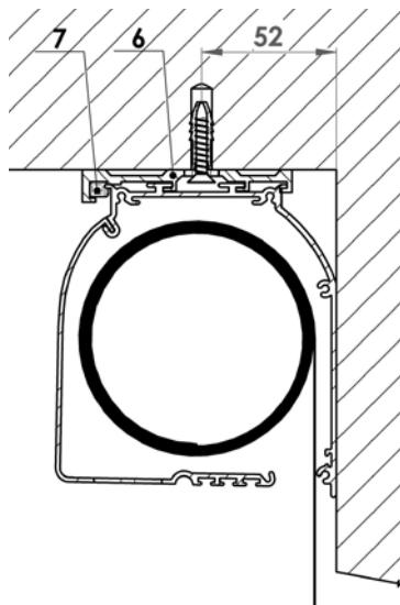
Attach brackets (6) using screws and components suitable for the type of structure onto which they are to be attached (metallic structure, window frame, wall, other material). If four brackets are used, ensure that the brackets are perfectly aligned  $\pm 1$  mm; this can be checked by sliding the box along the cut-outs before tightening the attachment screws.
