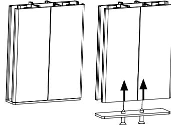
With Al end stops on the bottom part for the end stop of bottom rail; thickness 2 mm.
