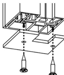
If the guide bars do not lean against the window sill or floor, end covers must be used. Before further installation steps, attach the cover by supplied screws.
