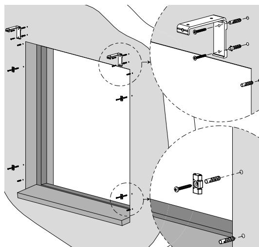
**Step 1: Drilling holes for the mounting brackets and guide rails**
