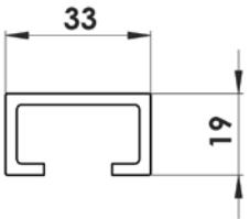
First, attach the box to the ceiling/wall, then install the guide rails. For model SCREEN LITE, only one type of guide rails is available – GC20. The bar is supplied with pre-drilled holes, as per order, from the front or from the side.
