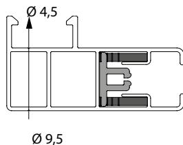
Guide rails for drilled openings on the front side:
