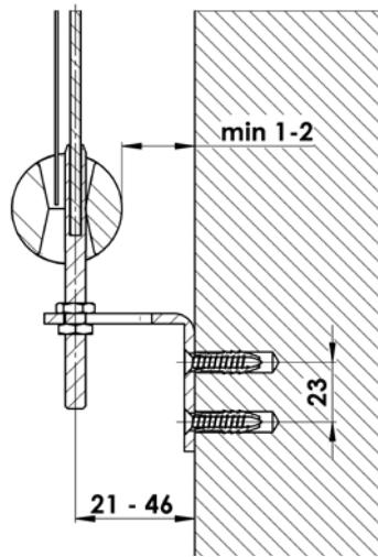
Lower brackets can be installed on the side or front, while the angle section aims down (a) or up (b).
