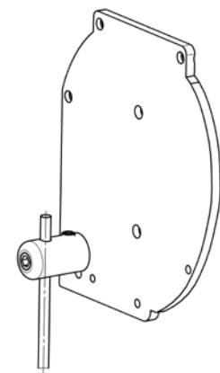
Attach the brackets to the wall using screws and components suitable for the type of structure onto which they are to be attached (metallic structure, cement, brick, etc.). If necessary, increase the bracket distance from the wall by washers. Always tighten the cord and hold it to prevent twisting.
