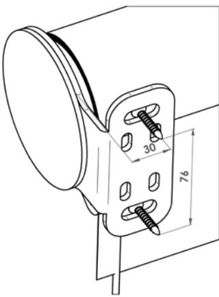
Start the screen roller blind assembly to the ceiling by marking out the attachment holes of the supporting brackets.
