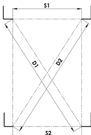
Once the installation is finished, check parallelism and rectangularity of the guide bars. This can be done by measuring two distances "S1" and "S2" or diagonals "D1" and "D2". The dimensions must be the same  $\pm 2$  mm. Proper guide bar placement is vital, otherwise the function of the roller blind can be impaired.
