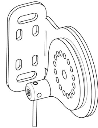
Attach the brackets to the wall using screws and components suitable for the type of structure onto which they are to be attached (metallic structure, cement, brick, etc.). A gap of 1-2 mm should be left between the lower section and the wall/window to prevent mutual damage during operation. If necessary, increase the bracket distance from the wall by washers. Always tighten the cord and hold it to prevent twisting.
