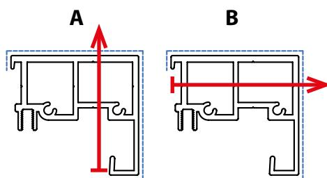
For model ZIP, only one type of guide rail is available – GC20. The rail is supplied with pre-drilled holes, as per order, from the front or from the side.
