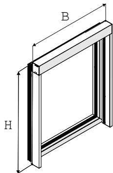
The dimensions to be specified are the width B and the height H. The finished width B is equal to the width of the box, which also corresponds to the distance between the outer sides of the left and right guide rails. This width is not always the width of the window, but depends on the window finish (see figure).
