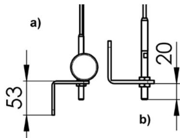
Lower brackets can be installed on the side or front, while the angle section aims down (a) or up (b).
