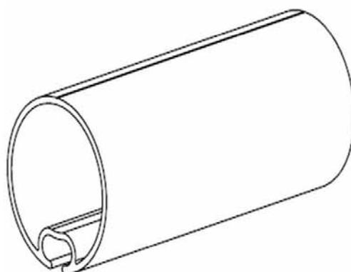
Material: Extruded aluminium (Ø40, Ø55 or Ø67 mm).
