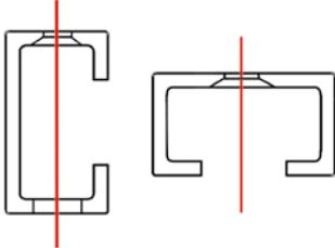
The red line indicates the vertical axis for attachment screws. Use the drilled guide rails as a template for transferring the hole positions to the window wing wall. Attach the guide bars to the wall using screws and components suitable for the type of structure onto which they are to be attached (metallic structure, cement, brick, etc.).
