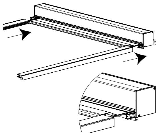
**Step 2: Sliding the guide rails over the console pivots on the bottom of the box**
