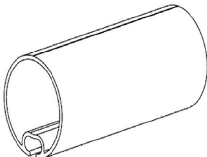
Material: extruded aluminium for tubes Ø 55mm and Ø 67mm and galvanised steel for tubes ø 85 mm a ø 100 mm.
