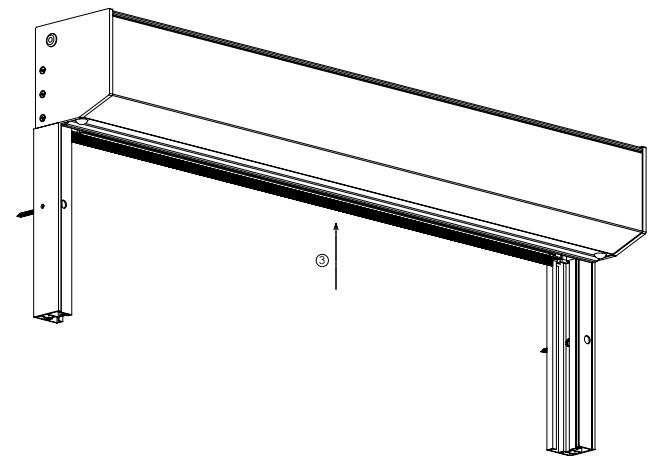
Insert the fabric into the guiding channels.
