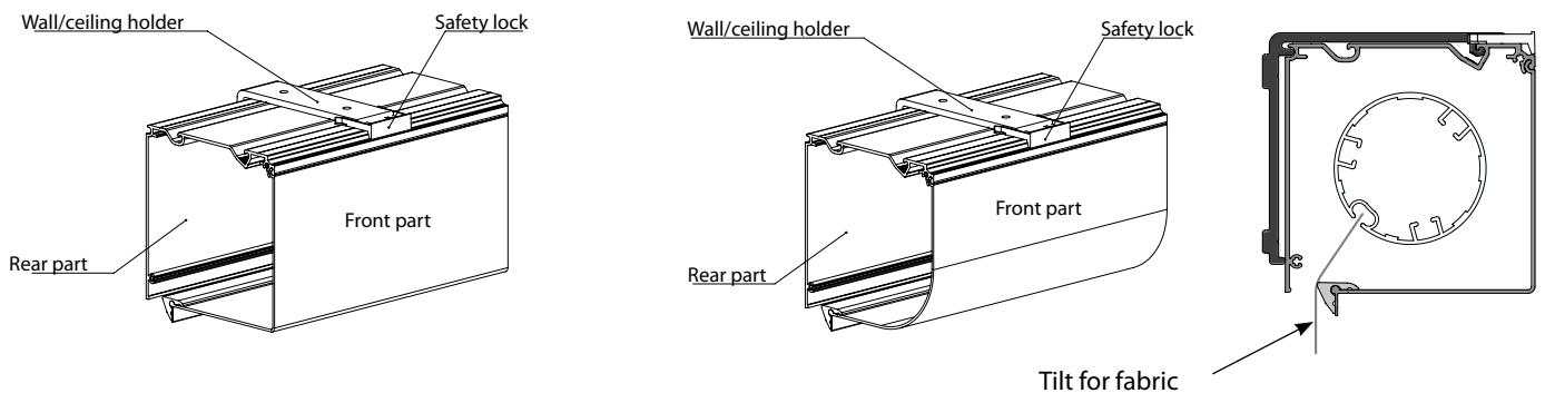
**Material:** extruded aluminium with powder coating finish
