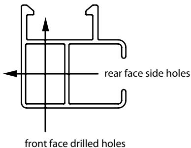
Guide rails for side and/or rear face drilled holes:
