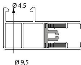
Guide rails for drilled openings on the front side:
