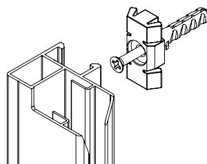
End stop on the auxiliary guide rail
