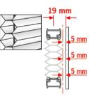
Push the lower parts of the tension shoe on the left and right into the recess on the side of the installation aid or press them in from below.
